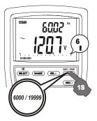
**MAX/MIN** Recording Mode: Press REC button momentarily to activate MAX/MIN recording mode. The LCD "R" & "MAX MIN" turn on. The meter beeps when a new MAX(maximum) or MIN(minimum) reading is updated. Press the button momentarily to read the Real-time, MAX & MIN readings in sequence. Press the button for 1 second or more to exit MAX/MIN recording mode. When activated, Auto-Power-Off is disabled automatically.
